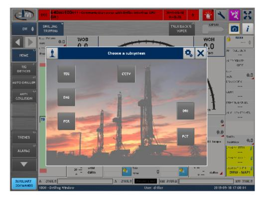
All the electrical and software sequences simulates the relative starting conditions and interlocks. It's possible to create failures related to the absence of those conditions, to be able to focus on reasons and corrective actions.
